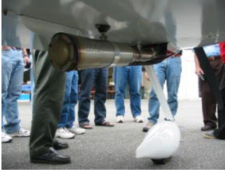
SuperTrapp exhaust reduced noise 50% with only 25 RPM reduction.
