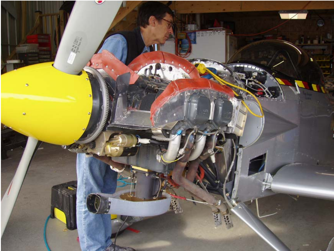
Bill Miller Scrutinizes the Electronics Bay of the Grenier RV-4-8 Note the “Piccolo tube” exhaust pipe exits - - -which give 3 Db noise suppression!
