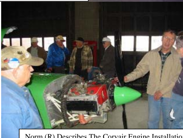
Norm (R) Describes The Corvair Engine Installation
